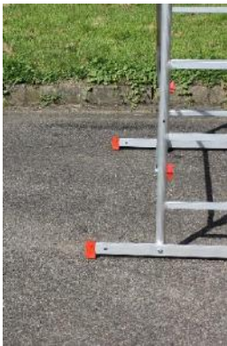
No Stiffener Bars and No Outriggers
